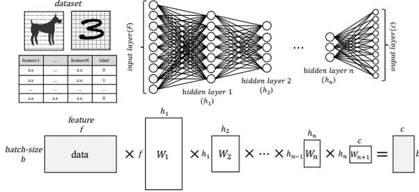
Fig. 2: Dense matrix multiplication application - Multi-Layer Perceptron classifier
