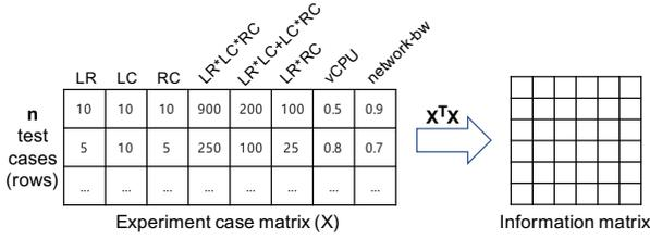
Fig. 9: Building an information matrix from experiment scenarios
