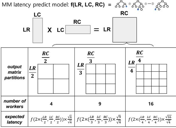
Fig. 8: Scaling-out prediction example
